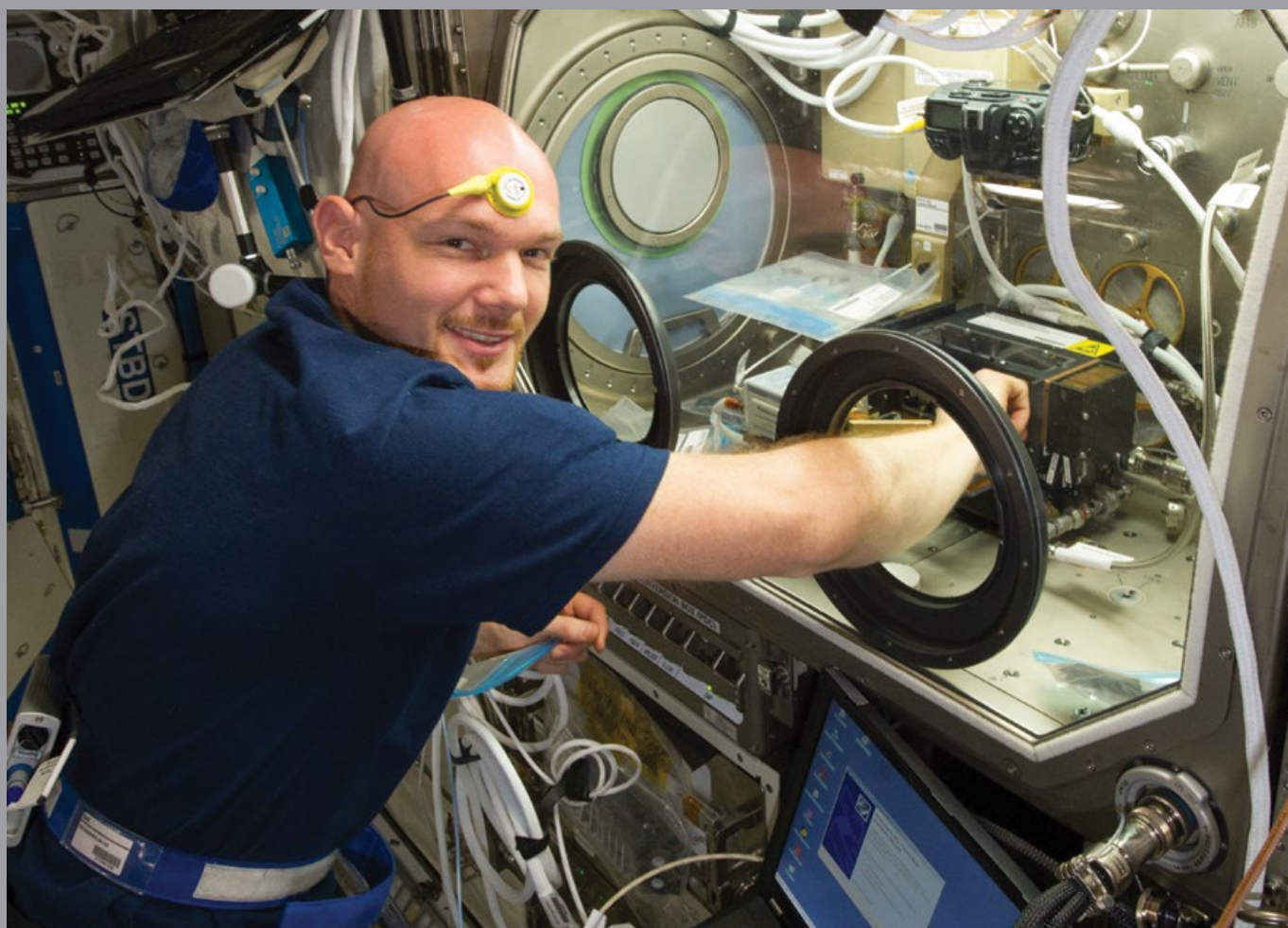
Alexander Gerst works with the combustion experiment known as the Burning and Suppression of Solids (BASS) in the Microgravity Science Glovebox in June. He is wearing a Dräger Double Sensor on his forehead for the Circadian Rhythms Experiment (NASA)
